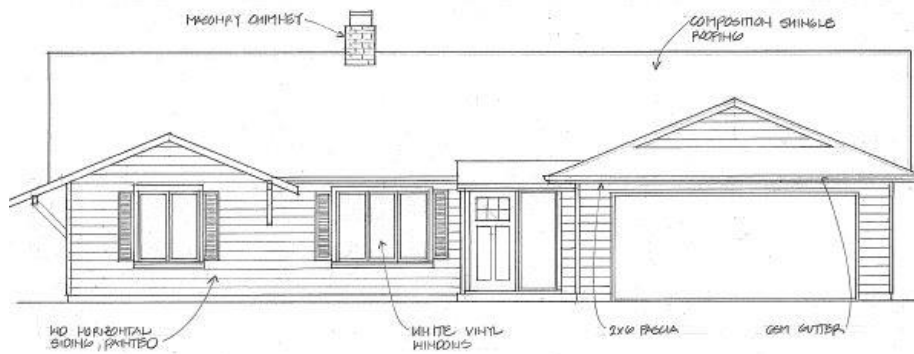
2 EXISTING EAST ELEVATION 1/8" = 1'-0"
